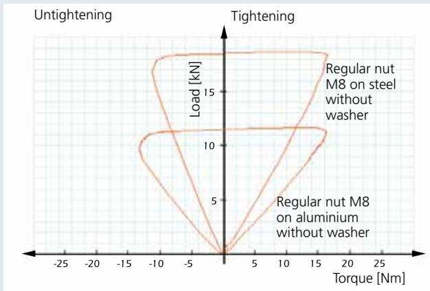
When no washer is used under the fastener, the friction depends on the contact surface. At a given torque, the obtained preload will vary depending on the contact material.
