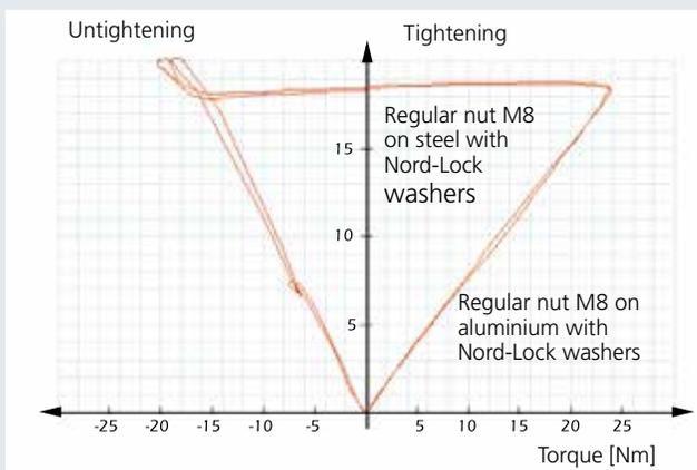
When using Nord-Lock washers, sliding always occurs between the upper washer and the bolt head / nut. At a given torque, the preload will be the same, regardless of the contact material.
