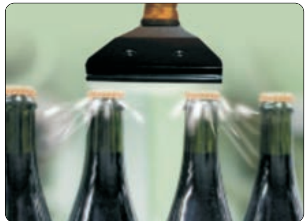
Air Edger™ Flat Jet with .008” gap setting blows water from under the caps on a bottling line moving at high speed
