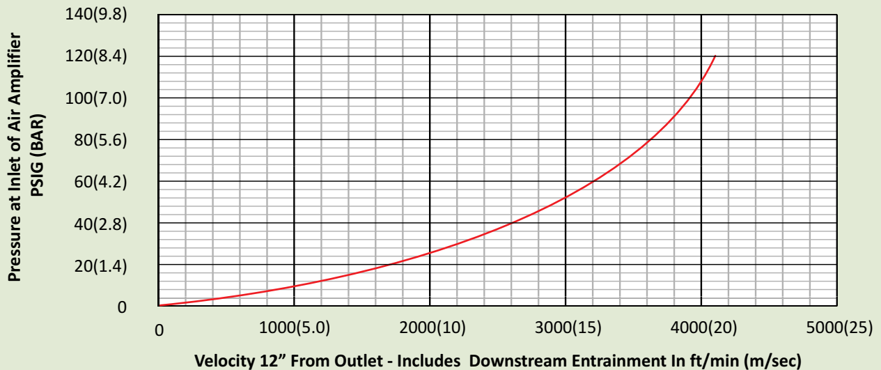
Pressure vs. Velocity 12" From Outlet for Model 40001, 40001G and 40001S Adjustable Air Amplifier
